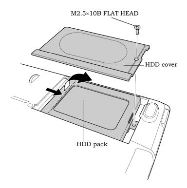
Figure 4-4 Removing the HDD cover
